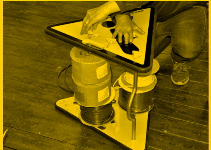
▲ Place cable drums on the bars, place top panel on top of bars, and secure using yellow nuts.
